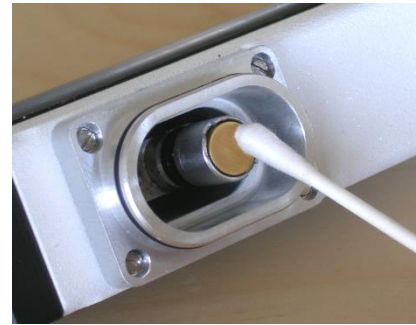
Fig. 5. Cleaning the transducer front.
