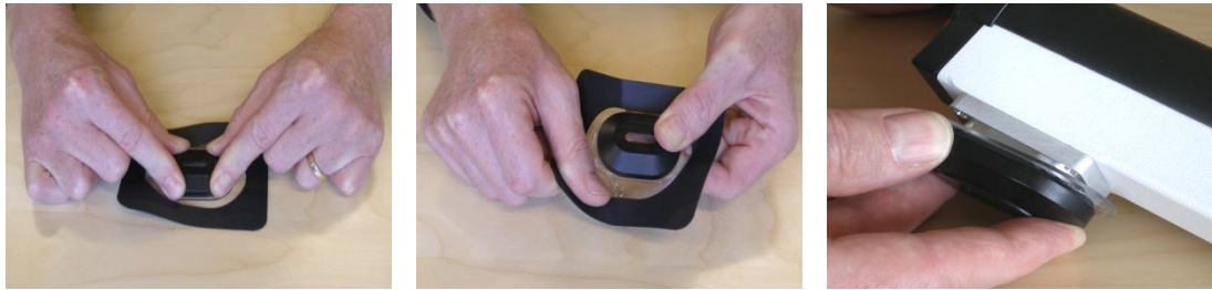
Fig. 2b. Mounting the water barrier.
