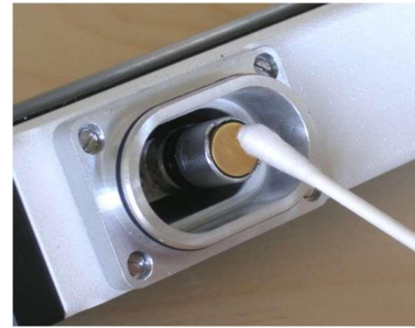
Fig. 5. Cleaning the transducer front.
