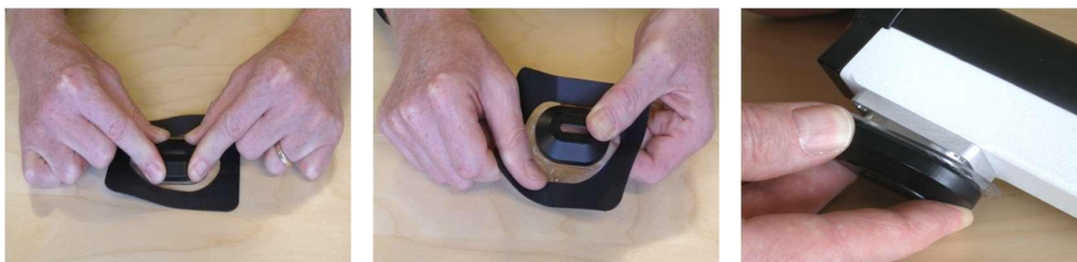
Fig. 2b. Mounting the water barrier.
