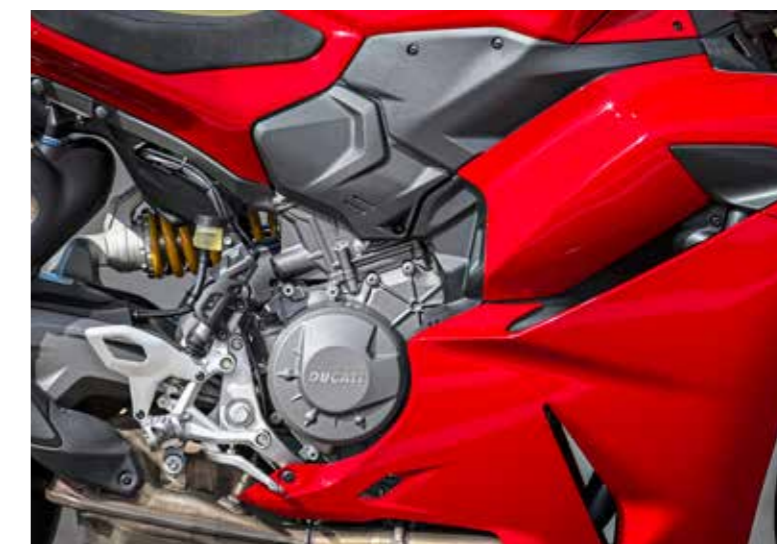
Chassis The V2 uses a cast aluminium mono-coque airbox frame. It features cut-outs for flex, weighs 4kg and uses the engine as a stressed member.
