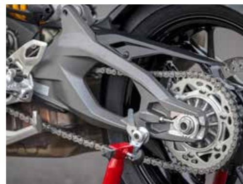
Swingarm It's out with the single-sided swingarm and in with a delicate V4 Panigale-style hollow aluminium double sider, for less weight and more lateral flex.
