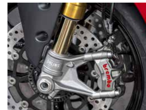
Brakes Brembo M50 four-piston monoblocs are brutally effective. ABS modes let you disable the rear ABS, or help you slide into corners.
