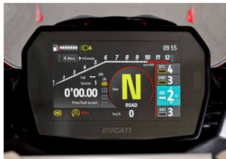
TFT New 5in colour dash has a 16:9 aspect ratio and three display modes: Road, Road Pro and Track, highlighting the relevant information you need.
