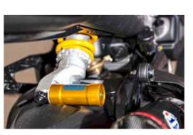
Top shelf suspension The new SP's fully adjustable Öhlins units provide a firmer set-up than the base Monster's preload adjustable rear shock and (0.6kg heavier) non-adjustable forks.
