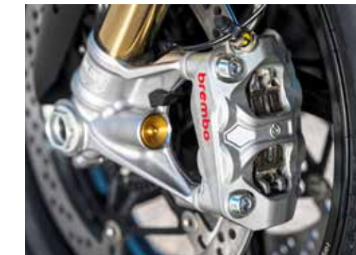
Brakes New Brembo four-piston Hypure calipers are lighter with improved ventilation. You can also spec them in red, yellow, black or gold.
