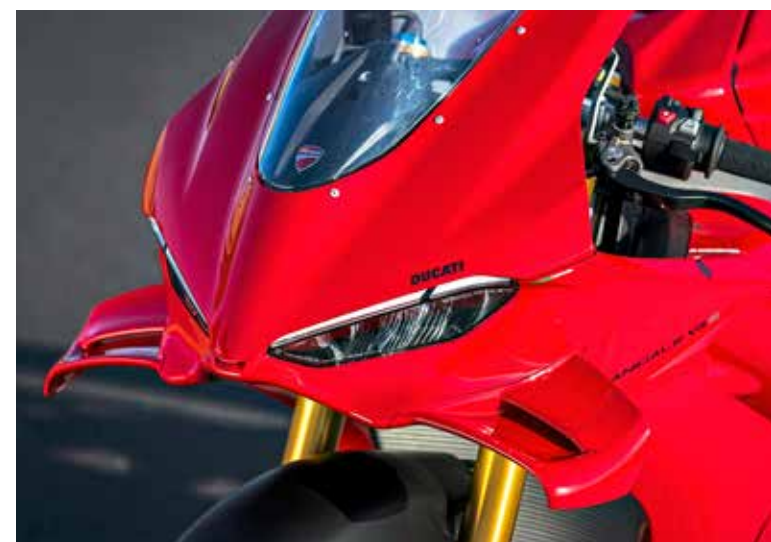
Aero New colour-coded wings create same downforce as before and integrate into the body. Fairing's leading edges are trimmed back to create less drag.
