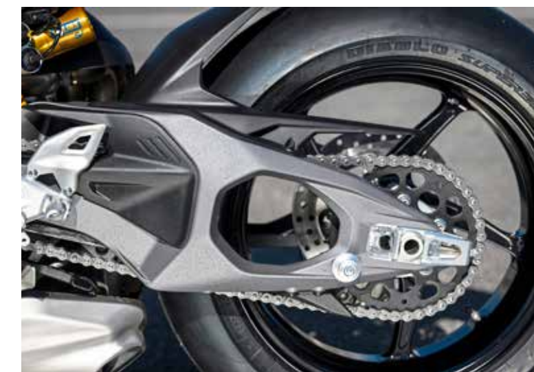
Lighter and more flexible double-sided swingarm and new frame are key to the Ducati's new-found ability to be easier to control, especially when grip fades.
