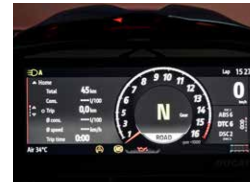
Dash Superb new 6.9in colour TFT has an 8:3 aspect ratio, cleaner new graphics and a plethora of easy-to-read information in road and track layouts.
