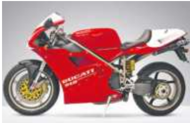
Ducati 955, 1996 ● 955cc ● 122bhp ● 182kg One of the rarest Ducati models ever, this machine was built purely to homologate the larger engine capacity for Ducati to take part in American AMA racing.
