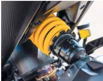
Preload adjustment on the rear and nothing up front but the suspension isn't lacking control in any way
