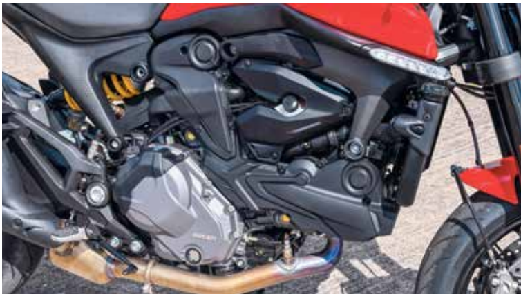
No trellis. Instead you have the front frame from the Panigale with the engine dictating the width – so end the result is gloriously slender
