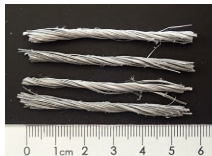
MasterFiber 320 “twisted” polyolefin macro fibers
