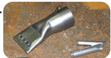
Speed weld attachment Correct hot air blower nozzle
