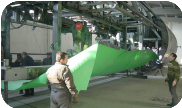
As secondary process, large collapsible forms (12m length) with AKS pulled tightly around outer perimeter.
