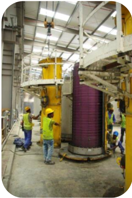
As secondary process, large collapsible forms (12m length) with AKS pulled tightly around outer perimeter.
