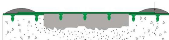
6. Then heat tack and temporary speed weld the overlap. Support the patch if required with ballast or formwork. The overlap should be min 30mm wide around the patch. Extrusion weld the patch to ensure a watertight seal.
