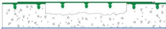
4. A new HDPE sheet is cut to the exact dimensions and inserted. This is Tack welded and speed welded in place
