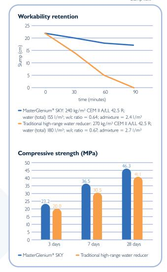
Removing 30 kg of cement can save over 20 kg  $CO_2$  emissions\*, while lowering the cost of the concrete.
