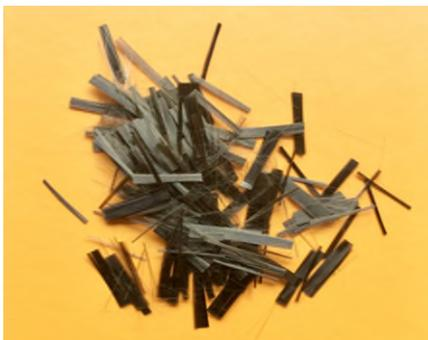
Micro fibre in basalto MasterFiber 050
