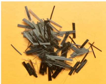
Micro fibre in basalto MasterFiber 050
