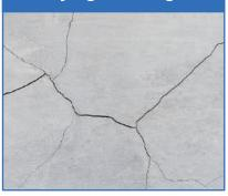
Environmental water loss due to drying of concrete
