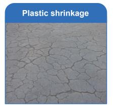
Water loss on concrete surface
