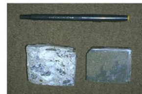
Steel dollies after testing. The rightmost dolly fails and shows insufficient bond. The leftmost dolly passes showing failure in the concrete substrate
