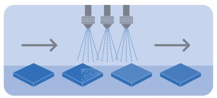
The MB-Pel SP products for surface treatment can be applied by sprayer or roller, either on the surface of the fresh elements, immediately after their compaction and stripping, or on hardened elements, after the curing stage.
