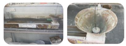
• The expected flow trough measurement for each Master Builders Solutions grout is given in the individual Technical Data Sheets.
