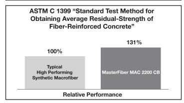
The new technology of MasterFiber MAC 2200 CB product has a unique combination of architecture and chemistry that provides superior performance compared to other commercially available synthetic macrofibers at an equal dosage. Alternatively, a lower dosage of MasterFiber MAC 2200 CB product can be used to achieve the specified properties, compared to typical synthetic macrofibers available commercially. The graphs above show the comparison between the
