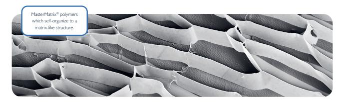
Developed by the experts from Master Builders Solutions®, MasterMatrix® products are customized viscosity-modifying agents (stabilizers and VMA) by which the right balance between high fluidity and high segregation resistance can be obtained.
