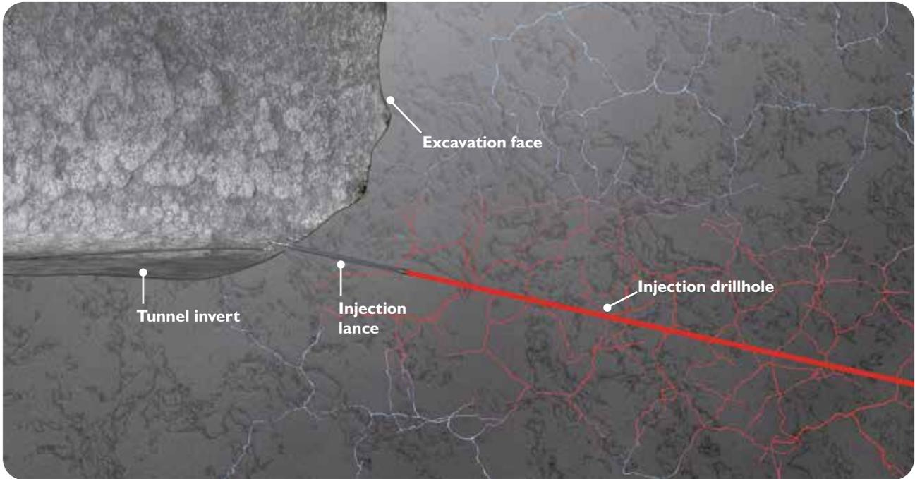
Stable microcement penetrating fine fissures
