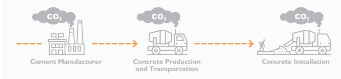
Embodied carbon: CO<sub>2</sub> associated with concrete production from the cradle to grave.
