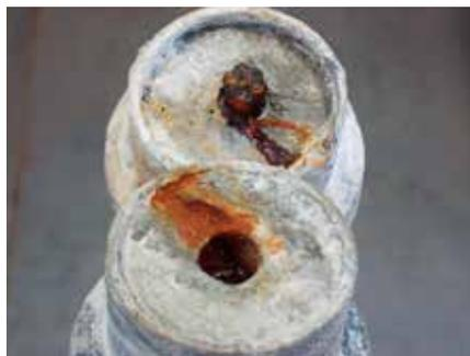
Without corrosion inhibitor
