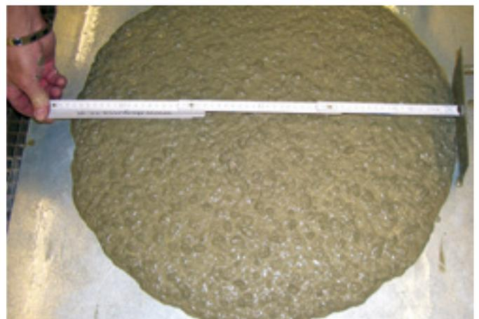
Sprayed concrete quality testing
