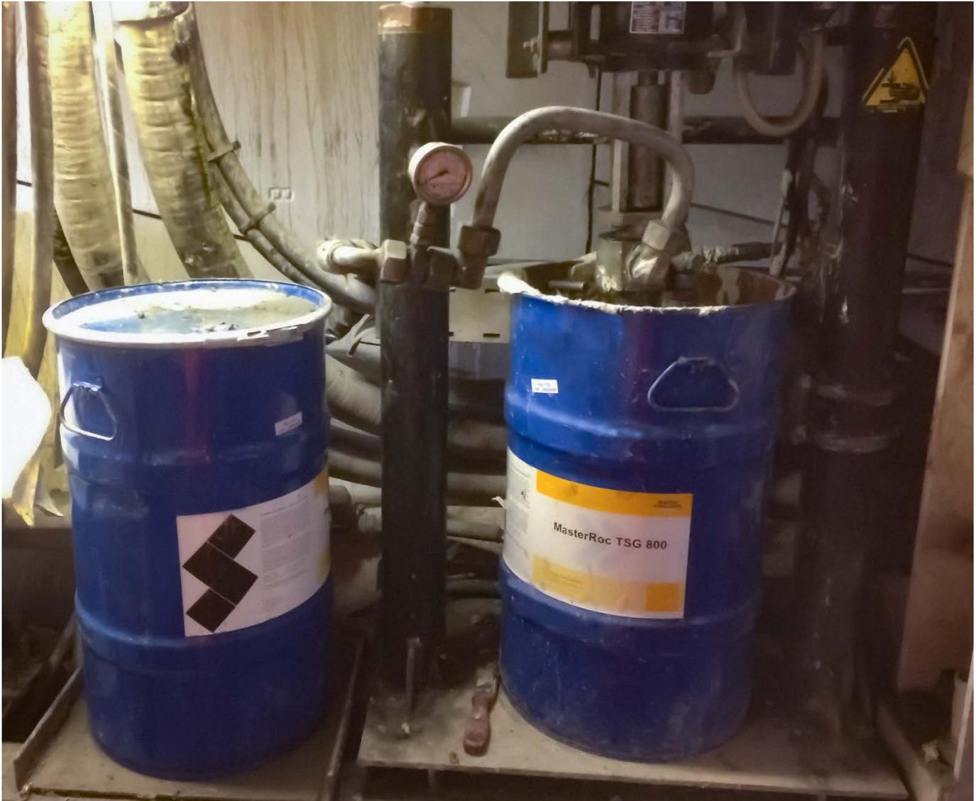
Reliable and cost-efficient sealing of the TBM tail shield is essential for a smooth tunneling operation. Regardless of the soil conditions and the annulus grout type used, the MasterRoc TSG tail sealants effectively prevent not only water but also soil and annulus grout from entering the TBM. Master Builders Solutions offers an inert tail sealant that does not produce any negative side effects for the concrete and the EPDM gaskets.
