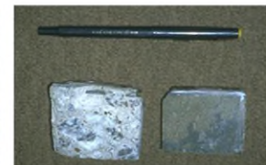
Steel dollies after testing. The rightmost dolly fails and shows insufficient bond. The leftmost dolly passes showing failure in the concrete substrate
