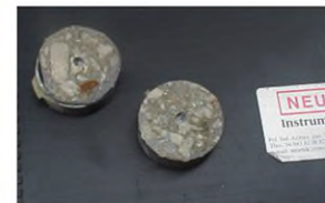
Steel dollies after testing. The rightmost dolly fails and shows insufficient bond. The leftmost dolly passes showing failure in the concrete substrate
