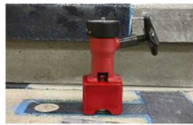
Direct tension loading device
