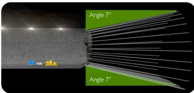
Pre-injecting approx. 24 meters into the rock ahead of the the tunnel face
