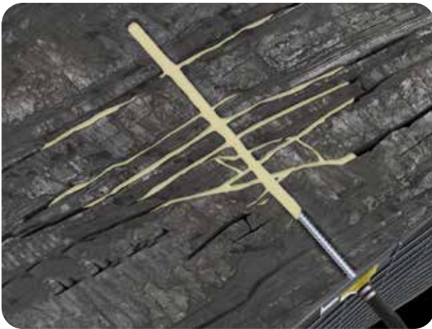
MasterRoc® RBA 380 fills cracks down to \geq 0.14 mm.
