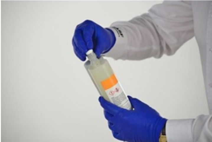
Figure 17 - Replace the white plug ensuring it is pressed home.
