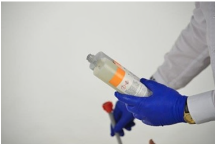
Figure 16 – Remove the static mixer and locking nut.
