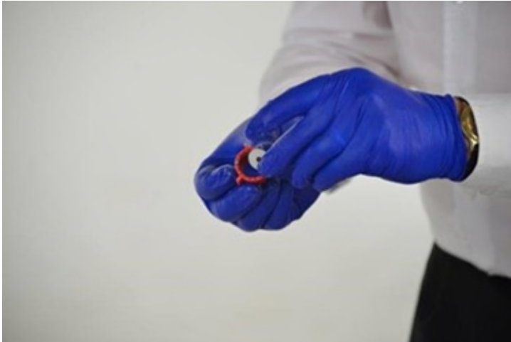
Figure 19 - Replace the metal washer in the red cap to secure the white plug.
