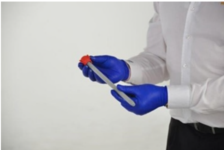
Figure 18 - Remove the red nut from the static mixer and discard the static mixer
