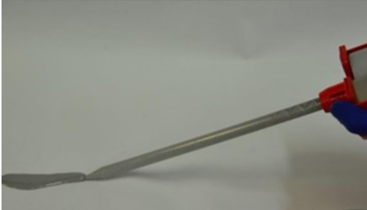
Figure 9 - The material will become a homogeneous grey colour by the time it is at the end of the nozzle and is now ready to use. Multiple cartridges can be gunned through one static mixer as long as the material has not gelled.
