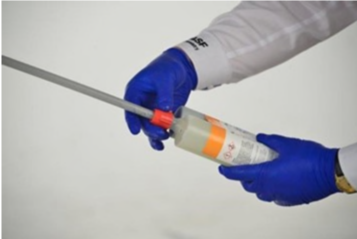
Figure 15 - Screw off the static mixer while holding the cartridge with the static mixer facing up
