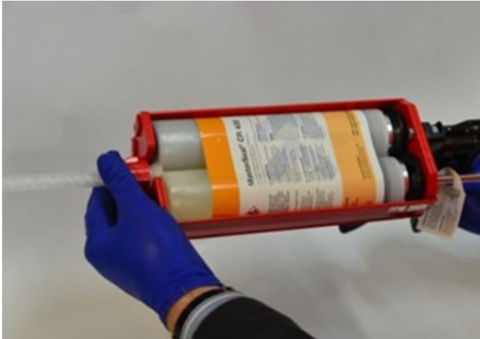
Figure 7 - Insert the cartridges into the gun ensuring the red cap is on the outside and the plungers are lined up with the cartridges.
