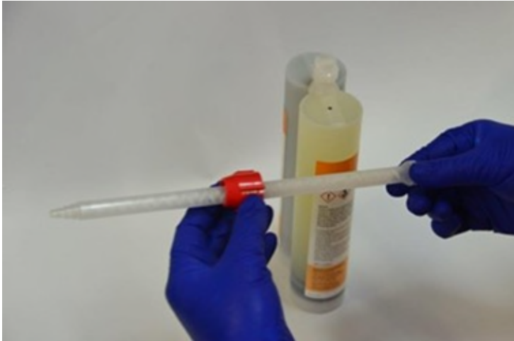
Figure 5 - Insert the static mixer into red cap and slide down to the thick end.
