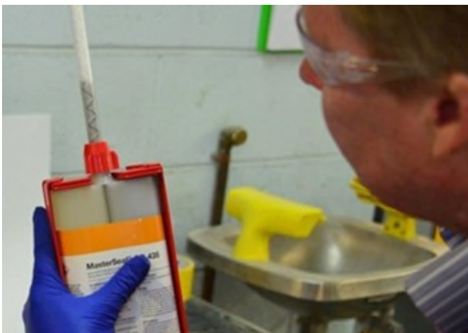
Figure 8 - Hold cartridges vertically to ensure any air in the cartridges is at the top and begin to extrude the material until it starts filling the static mixer. Note the reaction has started and the material in the static mixer will harden if left.
