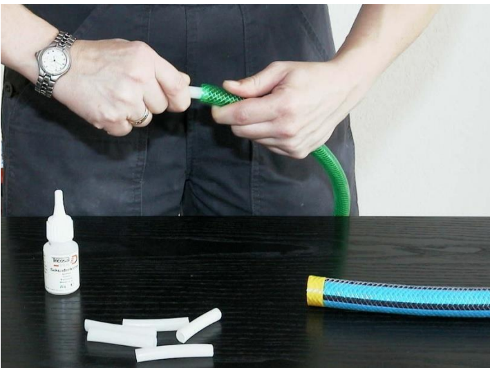
Figure 5: Insert connector after applying super glue
