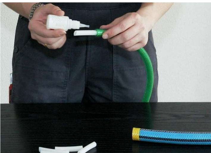
Figure 6: Put super glue on protruding section and insert inlet or outlet hose into the MasterSeal 909 hose
