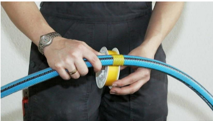
Figure 2: Wrap tape on hose to facilitate cutting
