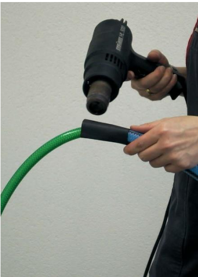
Figure 9: Use hot air gun to shrink sleeve to seal join
