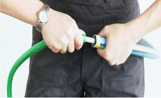
Figure 7: Put inlet and outlet hose together after applying super glue
