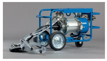
Example of a two-component injection pump.
