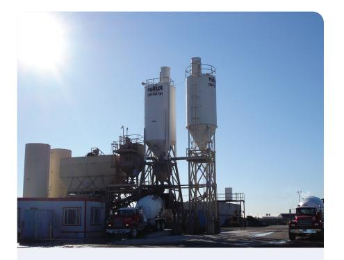
Portions of Interstate 80 at the Highway 505 intersection were in need of repair. The California Department of Transportation specified the use of "Rapid Strength Concrete" to minimize lane closures and disruption to traffic for these applications. The challenge during this project was that the concrete needed to achieve the required flexural strength even though the overnight temperatures were expected to be below freezing. **Project:** Interstate 80 and Highway 505 Lane Replacement
