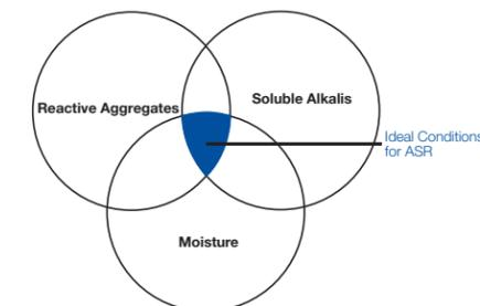
Figure 1. Conditions required for ASR
