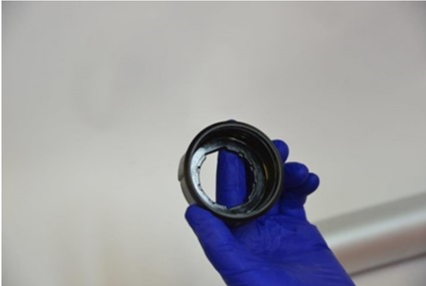
Figure 3 - Remove centre of cap if universal nozzle is to be used.
