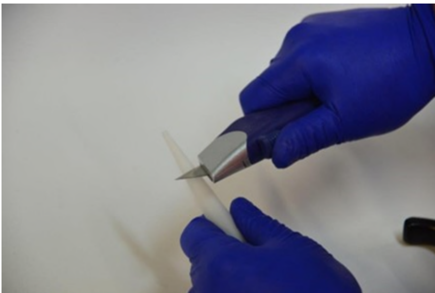
Figure 4 - Cut nozzle to 2-3 mm less than the width of the joint and at an approximate 45 degree angle.
