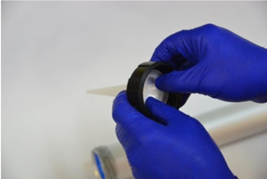
Figure 5 - Insert universal nozzle into cap and ensure it has snapped into place.
