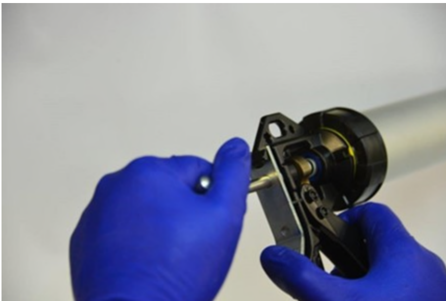
Figure 6 - Push on the catch plate to release the plunger and pull back to bring plunger back to the trigger end of the gun.
