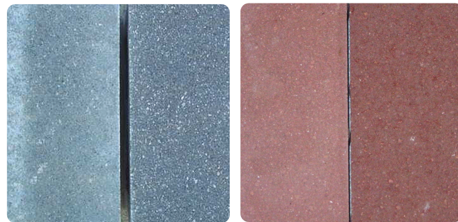
MasterPel 240 admixture-treated CMUs (right in each set) show reduced efflorescence and superior color vibrancy versus traditional water-repellent admixtures.
