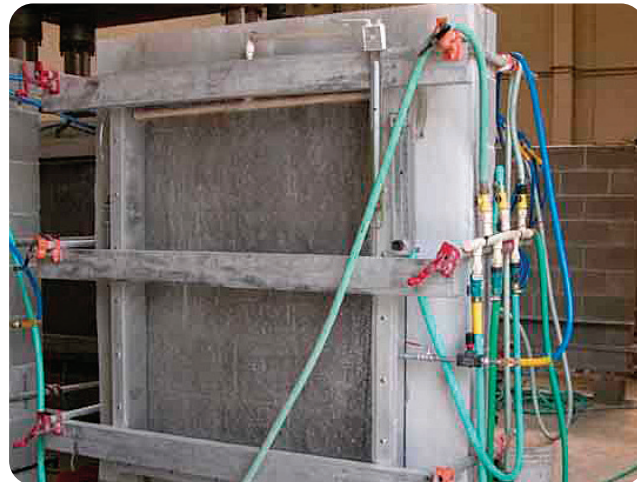
ASTM E 514 Testing of CMU wall
