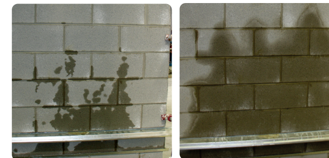
Project # 05-281 - Initial Testing Back of Reference Wall (no admixture)
