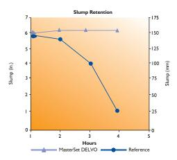
The graphs above are an example of what can be achieved through the addition of MasterSet DELVO admixtures to ready-mixed concrete.
