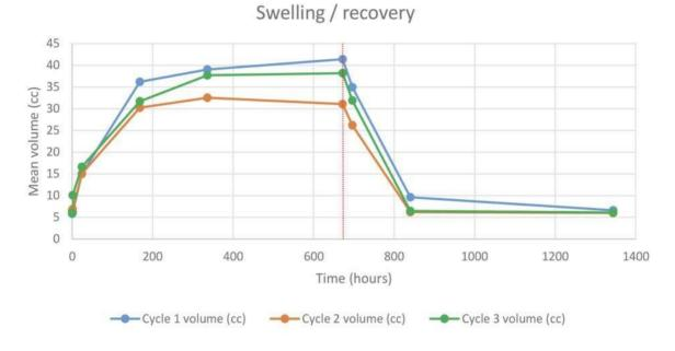
Note: The dotted red line indicates the end of the swelling and the start of the recovery cycle.
