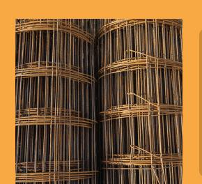
Light gauge welded-wire reinforcement (WWR) 6x6 W1.4xW1.4 152x152-MW9.1xMW9.1
