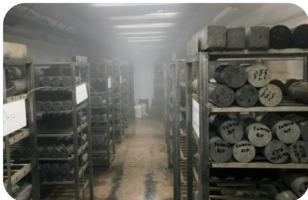
100% humidity storage, dry inner contents.
