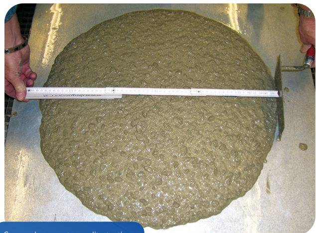
Sprayed concrete quality testing
