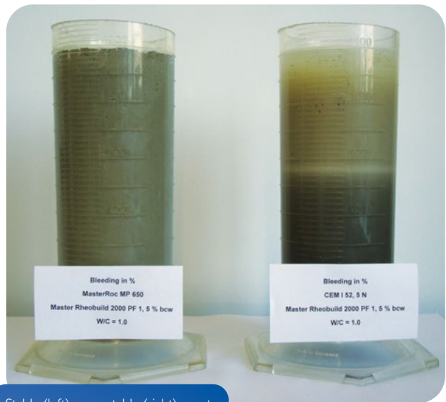
Stable (left) vs. unstable (right) grout
