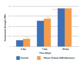
The chart (left) shows the effect that Master X-Seed I 500 has on the compressive strength of concrete.
