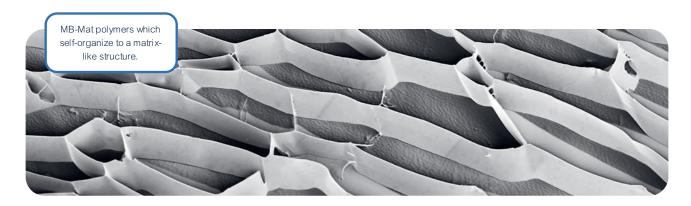
Developed by the experts from Master Builders Solutions, MB-Mat products are customized viscosity-modifying agents (stabilizers and VMA) by which the right balance between high fluidity and high segregation resistance can
