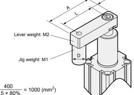
1. Calculate the required pressurized area.
