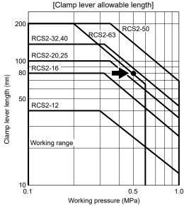
4. Confirm the allowable moment of inertia for the clamp lever.
