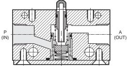
Note: Reverse-direction pressurizing (pressurizing from port "A") is not possible.
