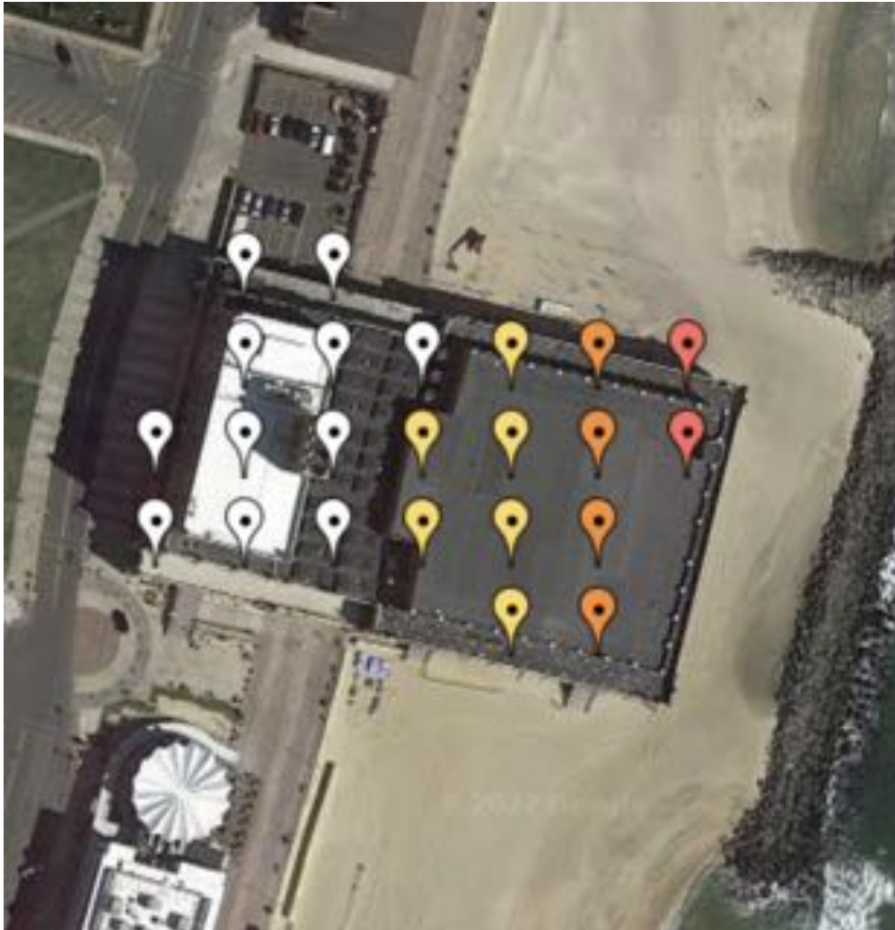
The land beneath elevated sections of the Asbury Park Convention Hall is projected to experience occasional to chronic flood risk by 2050. Yellow pins represent occasional flood risk; orange represents frequent risk; red represents chronic risk.
