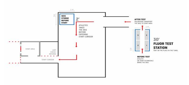
The place needs to be organized with 4 separate stations, each equipped by dedicated device (Bruker Alpha II) on slider system connected with separate computer. Only authorized persons may be present there.
