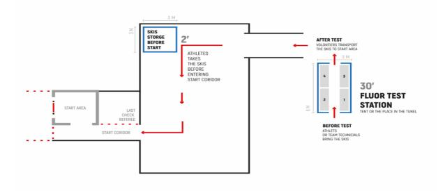
The place needs to be organized with 4 separate stations, each equipped by dedicated device (Bruker Alpha II) on slider system connected with separate computer. Only authorized persons may be present there.
