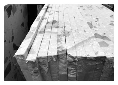
The raw edges of the slab are not smooth or square. We recommend that a 305x124 cm slab has a usable surface of 300x120 cm. Therefore, slabs will need to be processed offsite.
