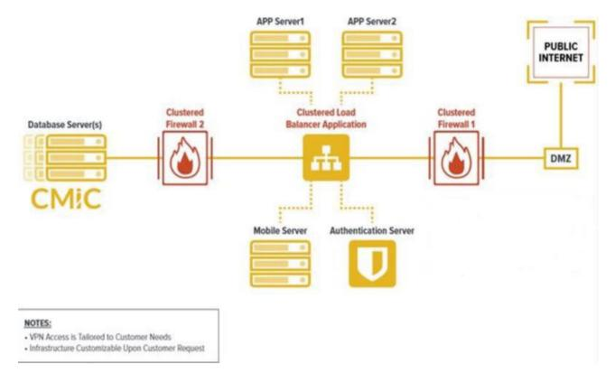
The infrastructure consists of servers, storage, and networking, with cloud-based security including but not limited to Distributed Denial of Service (DDOS) protection, web application firewall (WAF), and host-based threat protection.
