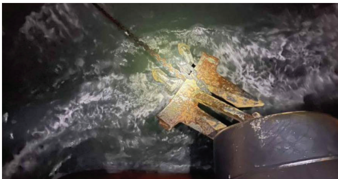
Anchor fouled with abandoned anchor and chain
