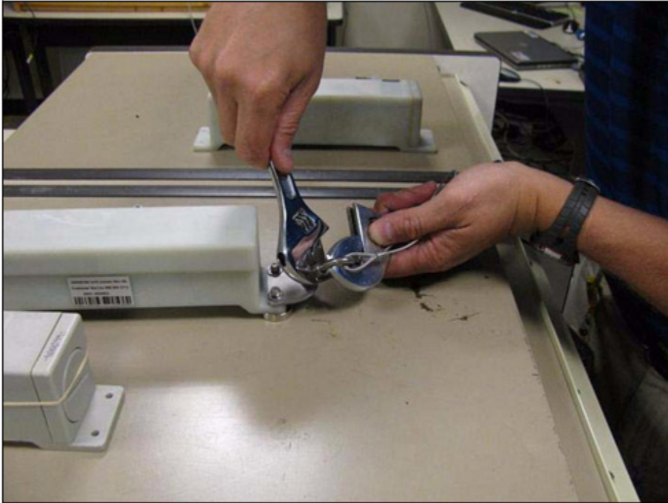
Figure 7 - Tightening the threaded link with two Crescent wrenches
