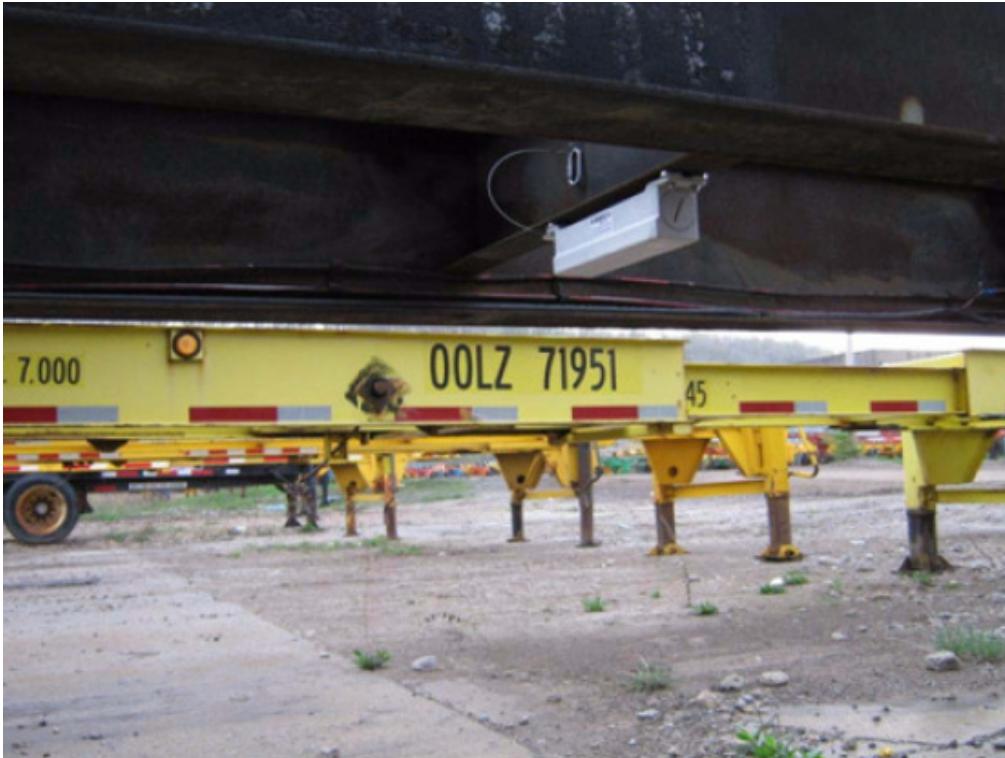
Figure 6 - Example of a mounted device centered side-to-side and front-to-back
