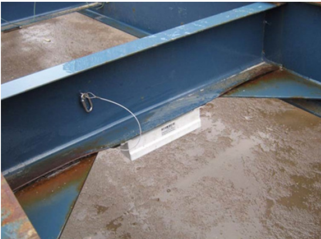
Figure 4 - Chassis mounting with the device facing down
