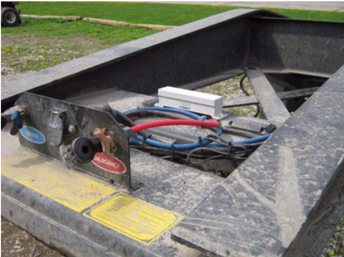
Figure 3 - Chassis mounting with the device facing up
